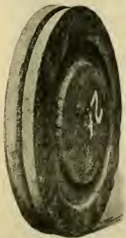
PAIR OF DISCS, AFTER FIRST FORGING.
